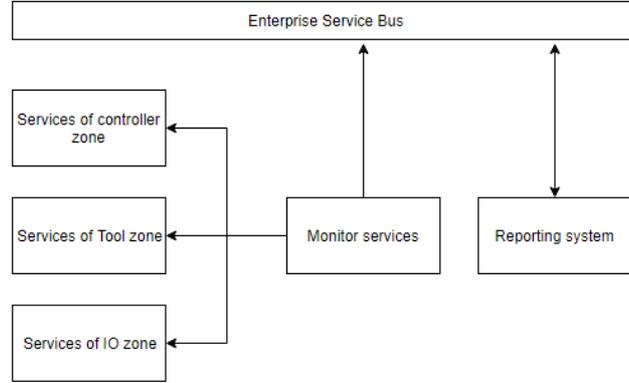
**Fig. 6.** The scheme of communication process between monitor services and other services in our platform.
