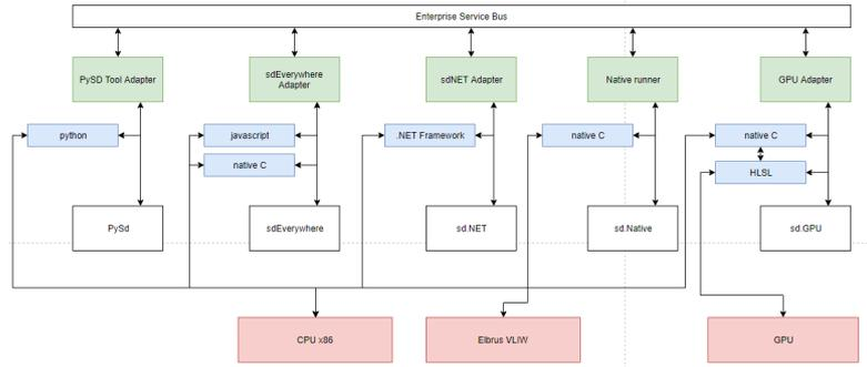
**Fig. 4.** The scheme of tool services dependencies upon technologies and platform types (green boxes – services, connected to ESB; blue boxes – technologies requirements for tool; red boxes – platform type requirement; white boxes – tools).
