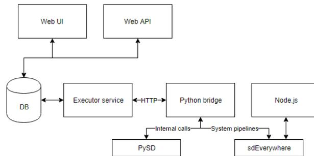
**Fig. 1.** The scheme of current architecture of sdCloud platform.
