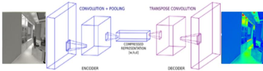
**Fig. 1.** The architecture of FCNN.
