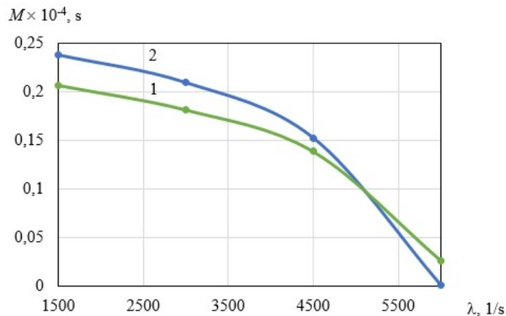
Fig. 4: The dependence of the efficiency criterion  $M$  on the intensity of packet arrival: with the multiplicity of the reservation  $K = 1$  (curve 1); with the multiplicity of redundancy  $K = 3$  (curve 2).
