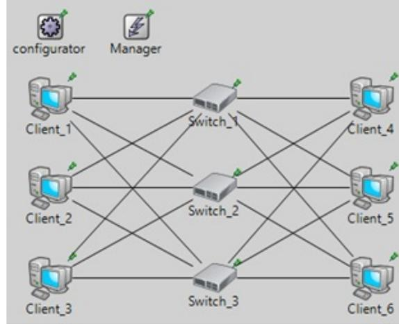
Fig. 2: The simulation model of the network with the possibility of the redundant transfers in the OMNeT ++ environment.
