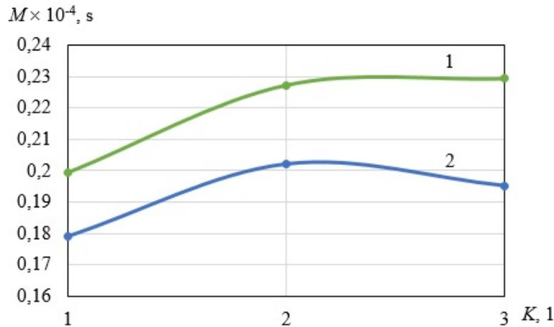
Fig. 3: The dependence of the efficiency criterion  $M$  on the redundancy ratio  $K$ : at an intensity of 2000 packets per second (curve 1); at an intensity of 5000 packets per second (curve 2).
