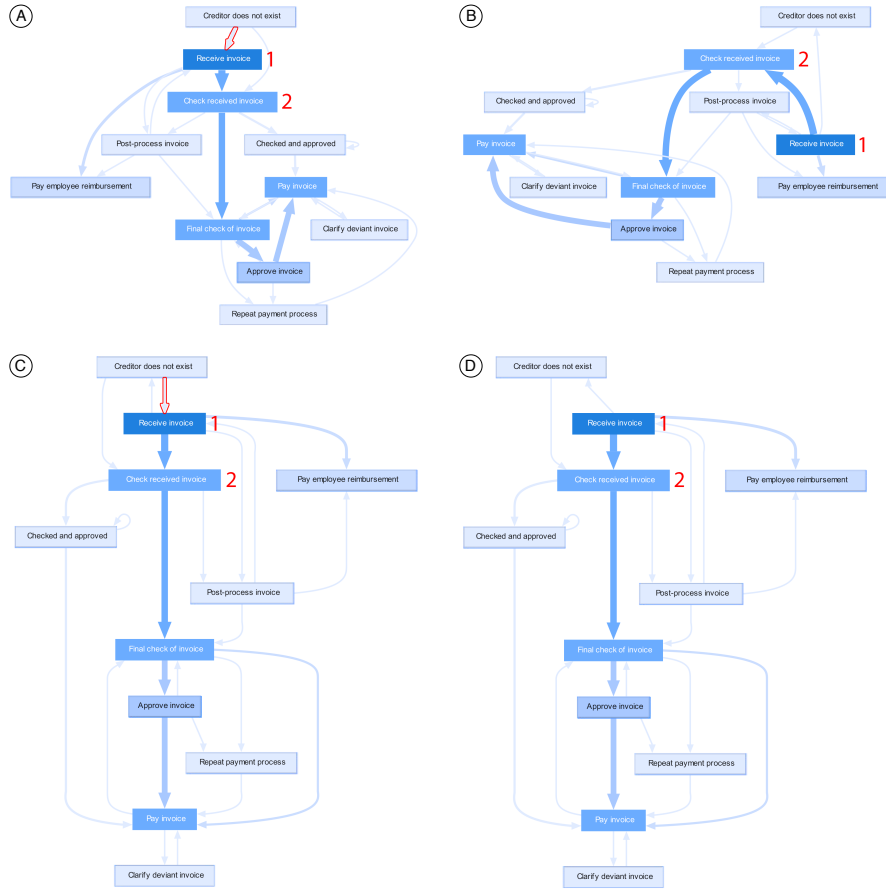
Fig. 1. Graphs A and B show the same process as graphs C and D, respectively. The layouts in A and B are computed by the industry standard [GKN15], where the actual process is poorly represented, while graphs C and D are computed by our novel graph layout algorithm where the process is easy to follow. Graphs B and D are obtained after removing the edge highlighted in red from A and C. As we can see, B differs significantly from A; especially note how nodes 1 and 2 swap vertically. Consequently, the mental map of the user is lost. On the other hand, C and D barely differ, preserving the mental map of the user.
