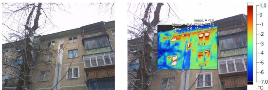
**Fig. 4** Photo and thermogram of the depressurization of the joint of the panels of the enclosure constructions
