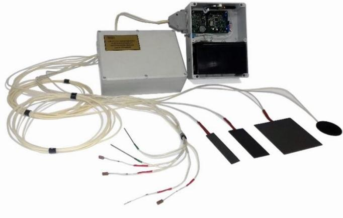
**Fig. 2.** Measuring modules of the thermal resistance monitoring system
