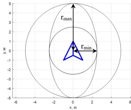
**Fig. 1.** UAV protection zone, inner circle corresponds to maximum turn rate in few seconds and outer circle characterized by cruise speed
