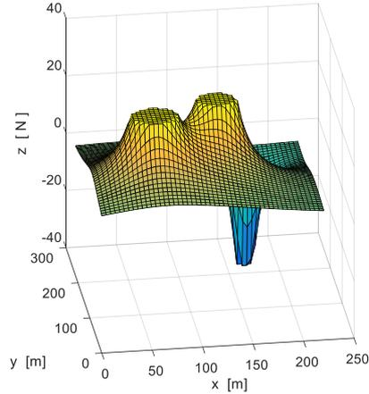
**Fig. 3.** Two obstacles and destination zone with high potentials formulate potential field
