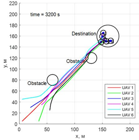
**Fig. 8.** Experiment 1. Flight trajectory of 6-th UAVs in a group with constant radius of protection zone
