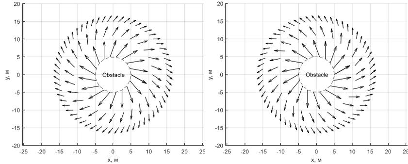
**Fig. 6.** Artificial vortex repulsion field is formulated around obstacle
