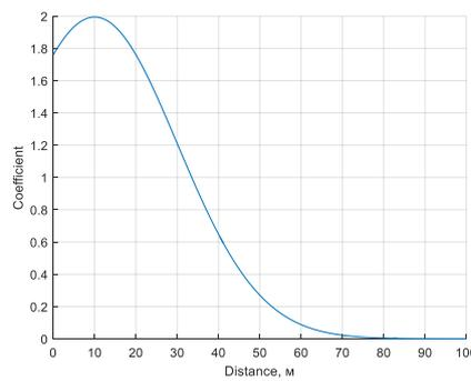
**Fig. 5.** Attraction force weighting coefficient dependence on distance to the destination
