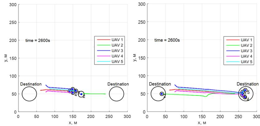
**Fig. 12.** Experiment 4. Collision avoidance with dynamic obstacle, like UAV with constant radius of protection zone around UAVs in a group and varying around standalone
