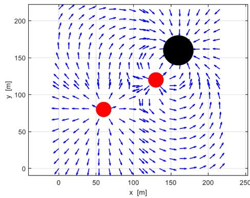
**Fig. 7.** Two obstacles and destination zone formulate potential field (red – obstacles, black – destination)
