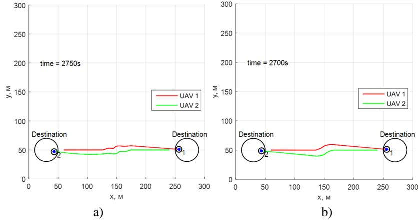
**Fig. 11.** Experiment 3. Collision avoidance with dynamic obstacle, like UAV with constant (a) and varying (b) radiuses of protection zone
