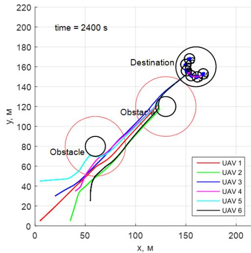
**Fig. 10.** Experiment 2. Destination zone is reached by 6-th UAVs in a group in 2400 seconds
