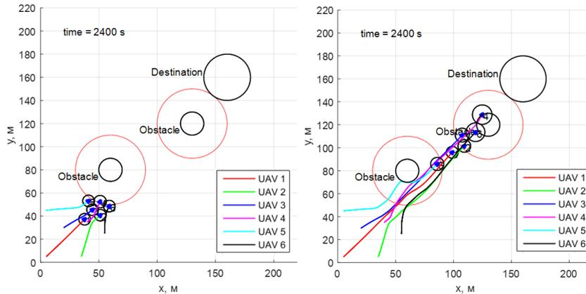
**Fig. 9.** Experiment 2. Flight trajectory of 6-th UAVs in a group with varying radius of protection zone
