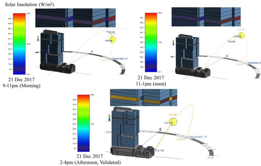
Figure 4: Solar Analysis Results at Different Times of the Day
