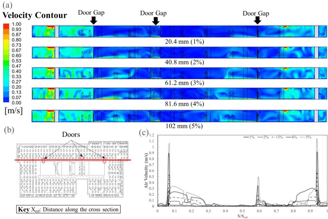
Figure 7: (a) Vertical Variations of Air Velocity for Different Door Gap Sizes in (b) Corridor; and (c) Comparison Different Door Gap Sizes among at the Height of the Centre of the Door Gaps
