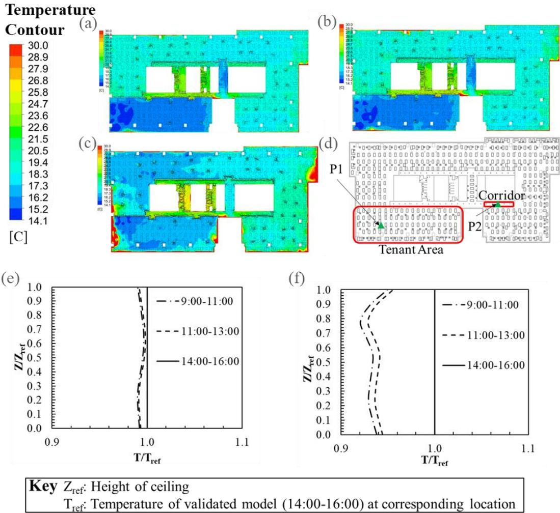
Figure 8: Temperature Distributions at Nose Level at Different Times of Day: (a) 9:00-11:00; (b) 11:00-13:00; and (c) 14:00-16:00; and Comparison of Normalized Temperature at Points Marked on (d) Floor Layout: (e) P1 in Tenant Area and (f) P2 in Corridor
