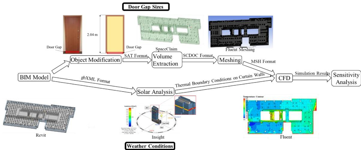
Figure 1: Workflow of Sensitivity Analysis using BIM and CFD
