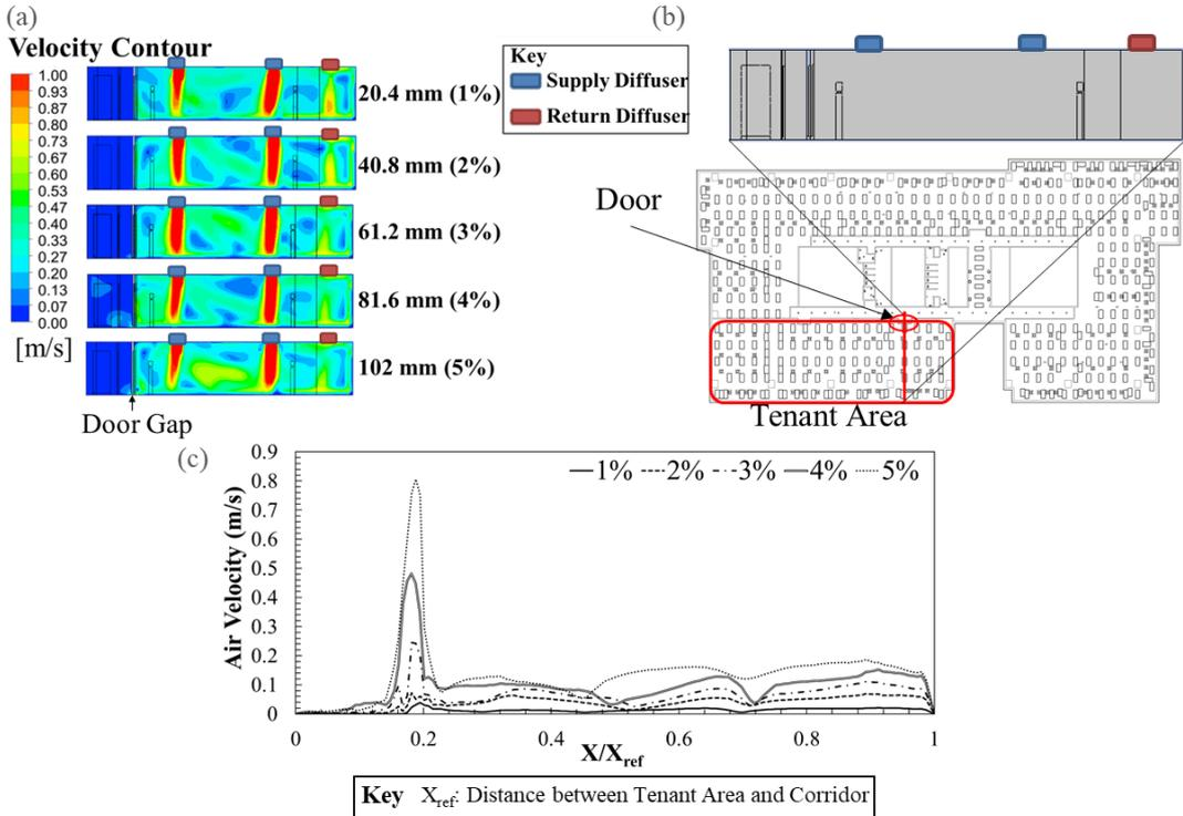
Figure 6: (a) Vertical Variations of Air Velocity for Different Door Gap Sizes in (b) Tenant Area; and (c) Comparison Different Door Gap Sizes among at the Height of the Centre of the Door Gap
