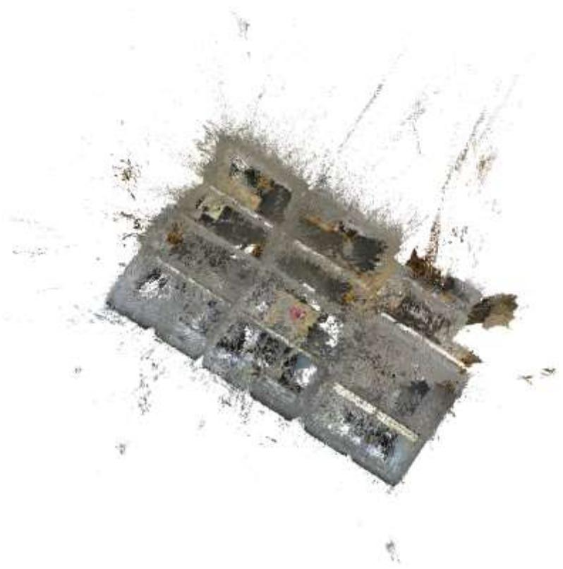
Figure 9: Reconstructed point cloud created through image matching. Point densities vary greatly with points scattered along their respective surfaces. Heavy noise and low point densities in regions such as the ceiling are quite characteristic.
