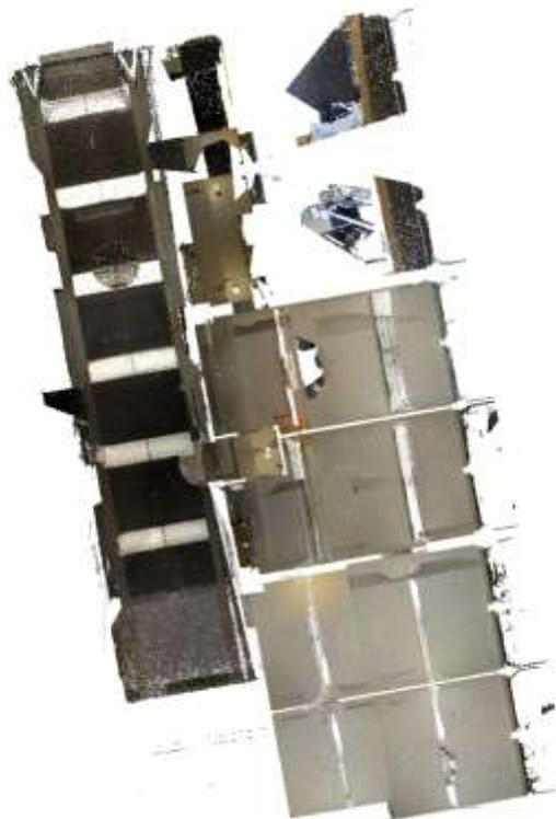
Figure 8: Point cloud reconstructed from multiple registered scans captured with a Riegl VZ400 laser scanner. The overall resolutions is very fine, but suffers from density fluctuations close to the scan positions.
