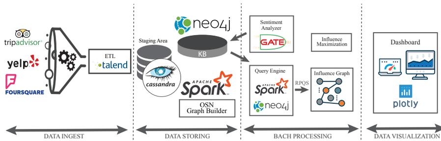
Fig. 3: System Architecture.
