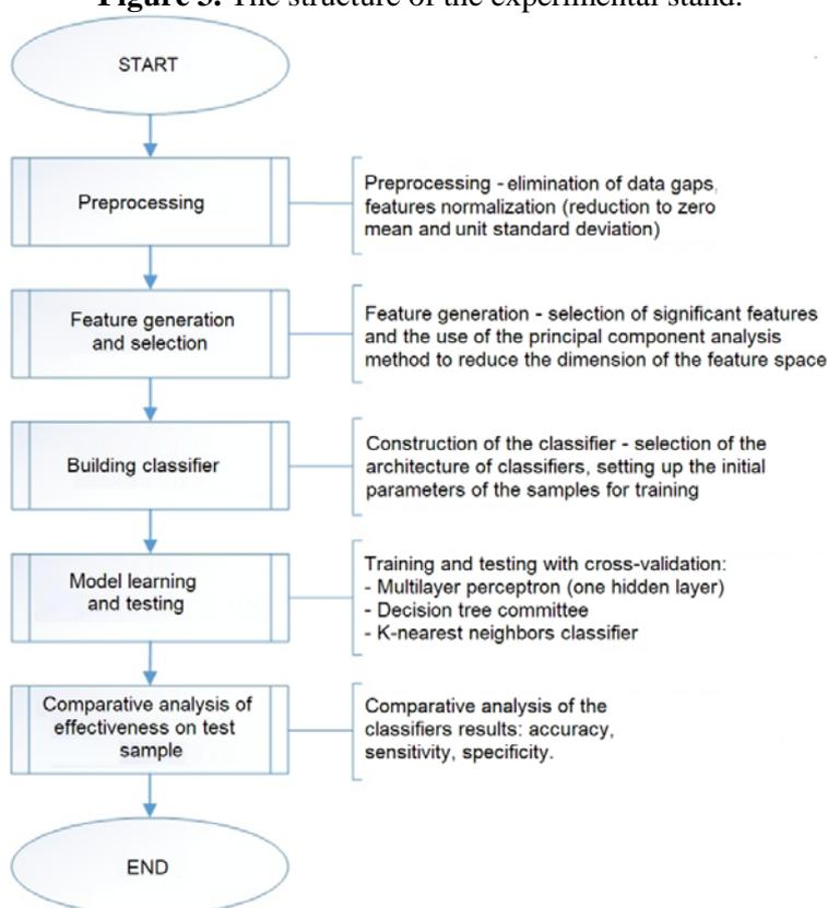
**Figure 4.** Flow chart of network traffic analysis.
