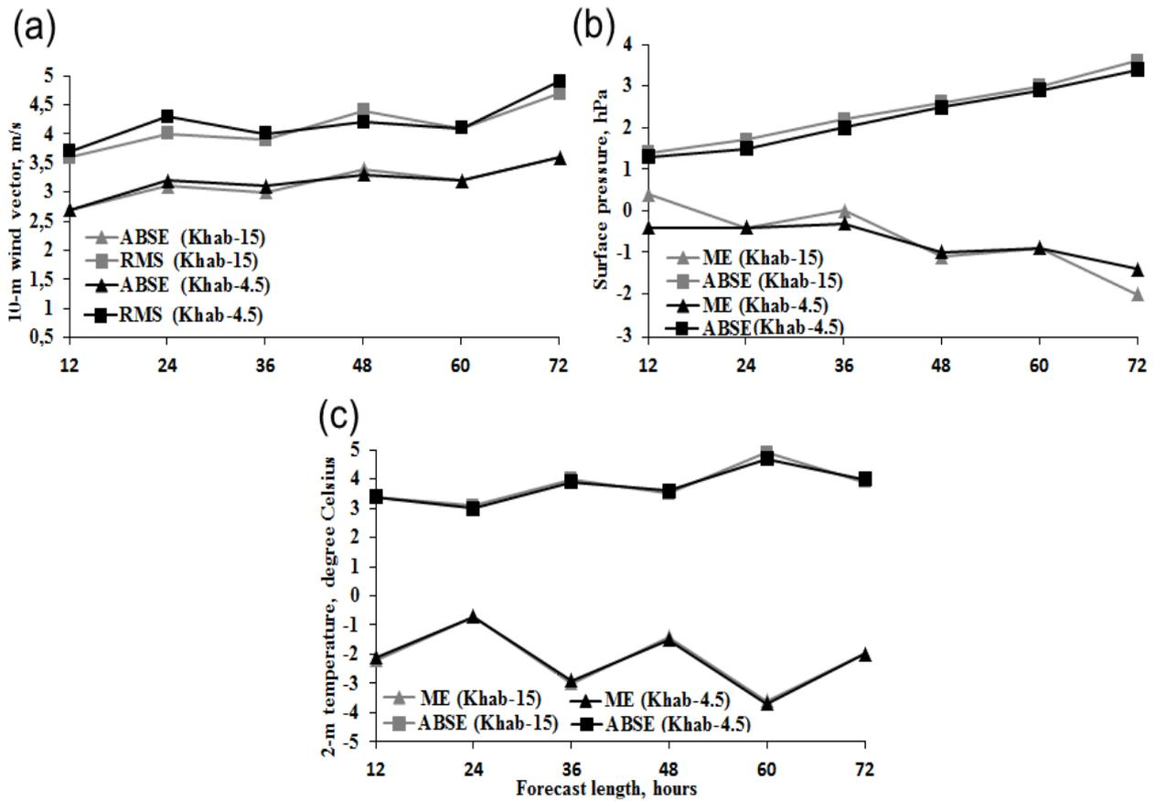
Figure 3: The accuracy of surface forecasts of NWP systems 'Khab-15' (grey) and 'Khab-4.5' (black), (a) 10-m wind vector (m/s), (b) surface pressure (hPa), (c) 2-m temperature (degrees Celsius) for the period of time from 14 January to 14 April, 2019
