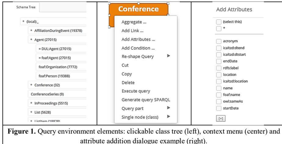
**Figure 1.** Query environment elements: clickable class tree (left), context menu (center) and attribute addition dialogue example (right).
