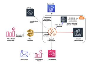
Fig. 1. Blueprint cloud architecture for consuming Neptune's CDC stream. Solid lines represent mandatory, dashed lines optional components.
