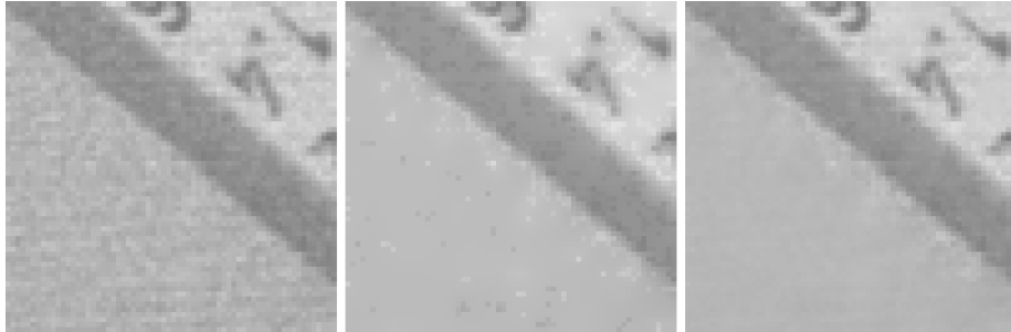
Fig. 1. Original image detail (left), remaining impulse noise in the unmodified method (middle), processed with the proposed method (right).
