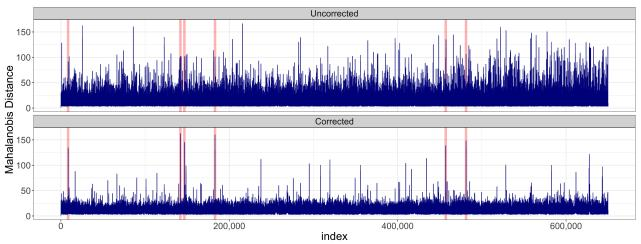
Figure 2: Mahalanobis distance over an ECG time series, before and after the window-based error correction method is applied.
