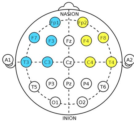
Figure 4: Electrode configuration
