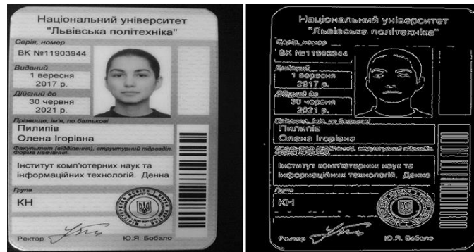
Fig. 7. The result of Canny algorithm
