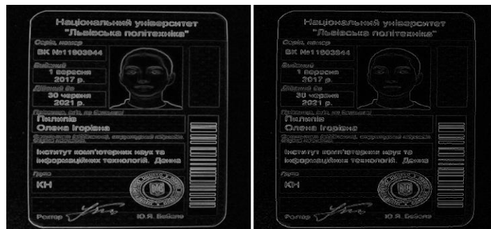
Fig. 5. The result of non-maximum suppression
