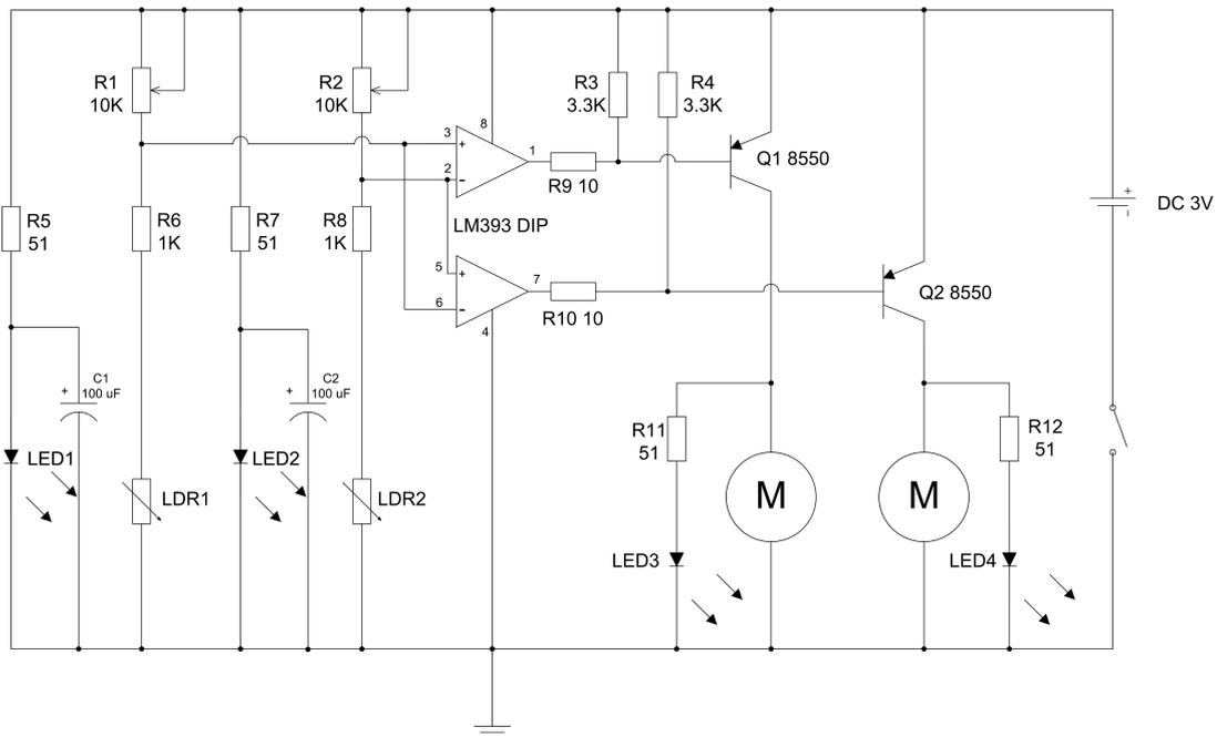
Figure 1: Circuit diagram of the line-follower robot based on LM393 dual differential comparator
