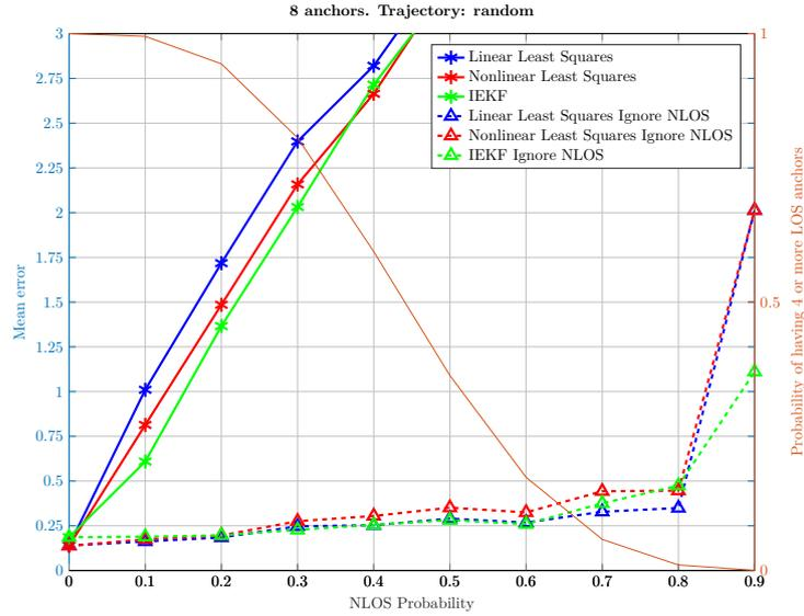
**Fig. 2.** Mean error of position estimates vs NLOS probability with a random trajectory. Right-hand side ordinate axis: probability of at least four anchors with LOS propagation conditions.
