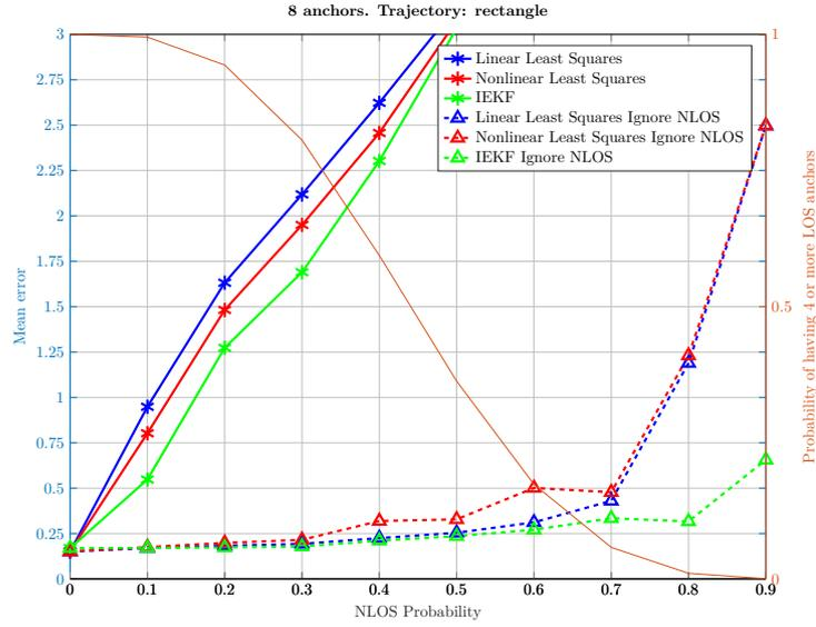
**Fig. 1.** Mean error of position estimates vs NLOS probability with a rectangular trajectory. Right-hand side ordinate axis: probability of at least four anchors with LOS propagation conditions.
