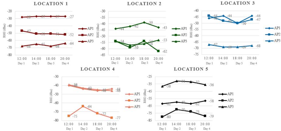
**Fig. 4.** Measured RSSI values from five different locations over four days indicating the fluctuation experienced in RSSI values
