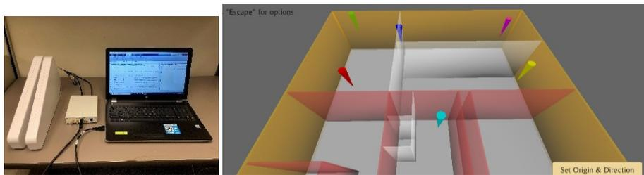
**Fig. 3.** Left: Each USRP set (one UE) includes a laptop and antennas for additional gain; Right: Screenshot of OTA indoor field test result integrated with BIM-IL portal, the white colored dividing walls are absent in the test, the dark blue and purple icons are anchor UEs, the light blue UE is purposefully set in an adjacent room separated by a wall so line-of-sight path is completely blocked from all other UEs.
