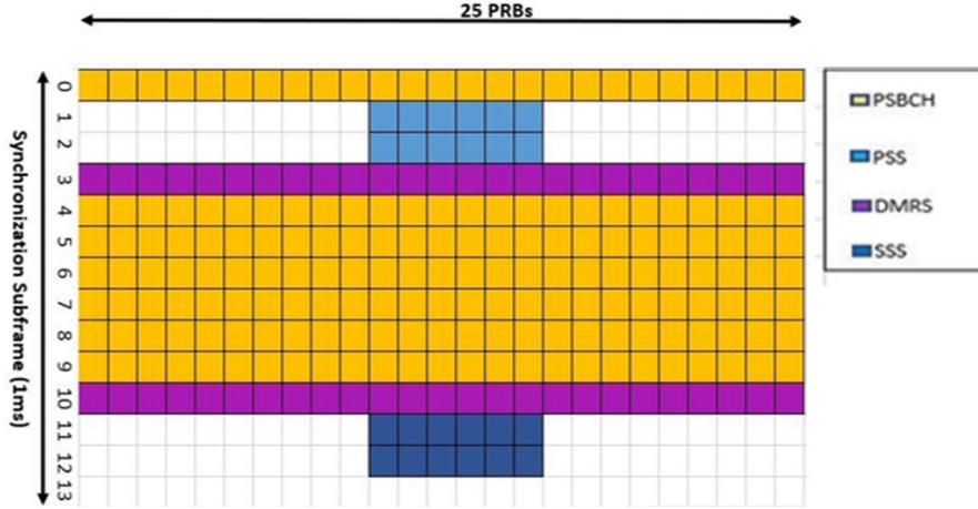
Fig. 1. Synchronization Subframe resource block structure of LTE SL air interface, 5 MHz mode. Vertical coordinate: time, horizontal coordinate: frequency.
