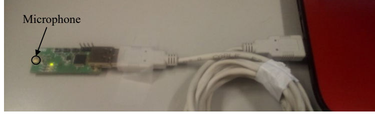
Fig. 2. Microphone-based receiver connected to a laptop that processes the ultrasonic information.
