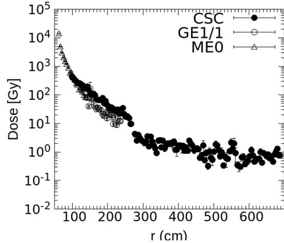
Figure 5. CMS Phase 2 simulation – combined dose at  $3000 \text{ fb}^{-1}$
