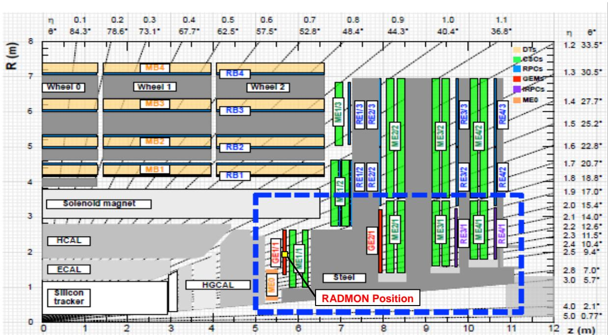
Figure 1. Transverse section of the CMS detector showing the present muon system. The RADMON was installed with a test GEM chamber in the free inner endcap station GE1/1
