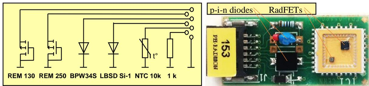
Figure 2. RADMON PCB: Schematics (left) and Photo (right)
