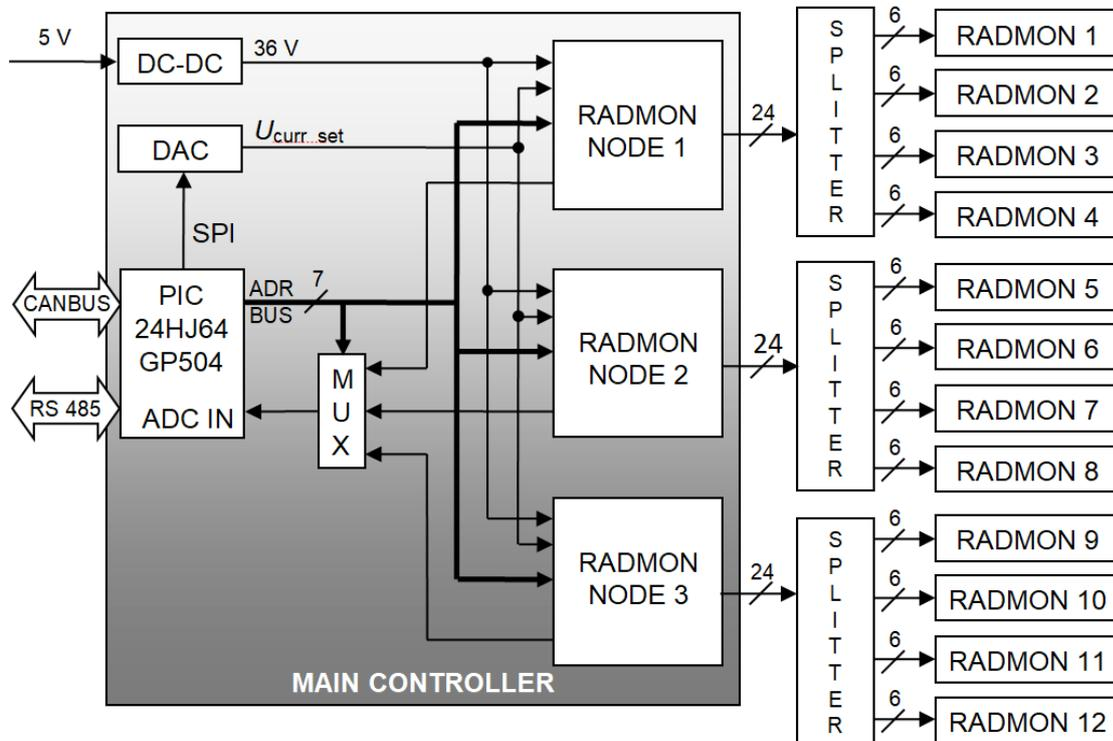
Figure 3. Block diagram of the RADMON Control and Read-out System
