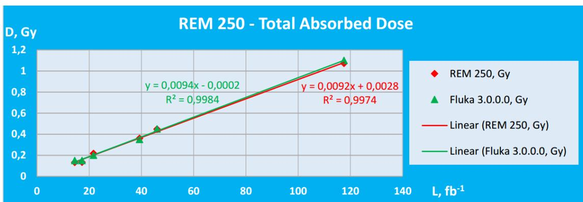
Figure 6. Experimental and simulated data for the total absorbed dose around Slot 1 of GE 1/1
