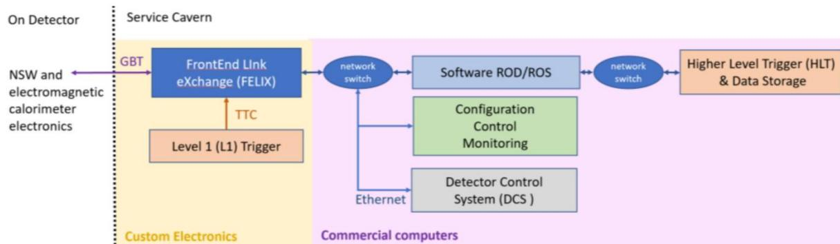
Figure 1. The upgraded ATLAS readout system. Data is routed by a custom designed FELIX board and software from the front-end detector electronics onto commercial computers. The commercial computers contain software to perform the data processing in the Software ROD/ROS, as well as detector control, monitoring, configuration, High-Level Trigger and Data Storage
