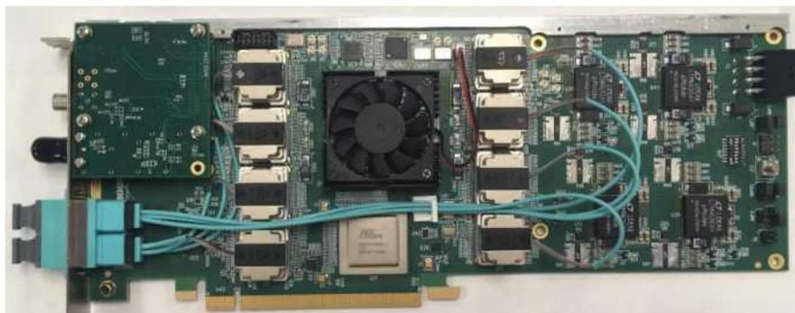
Figure 2. The FELIX card (FLX-712) showing eight miniPODs and the TTC mezzanine card with the fan-cooled FPGA
