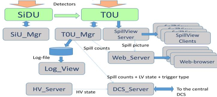
Figure 2. Software architecture for the BM@N experiment trigger system
