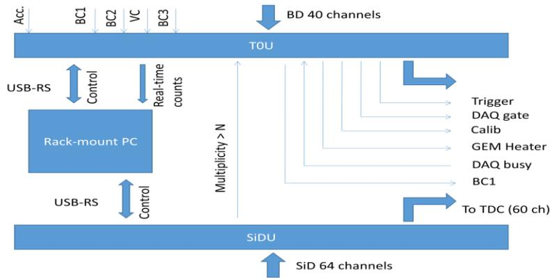
Figure 1. Configuration of trigger units for the BM@N experiment
