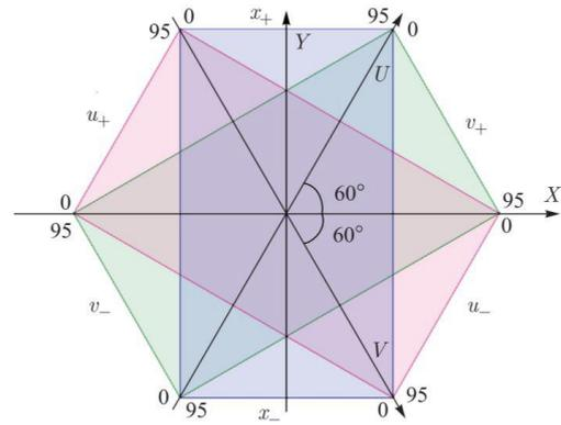
Figure 3. Coordinate system of the MWPC detector [6]
