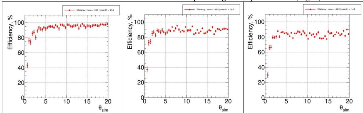
Figure 6. Efficiency of track reconstruction for 1, 2 and 3 particles in event
