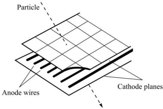
Figure 2. Structure of the MWPC detector
