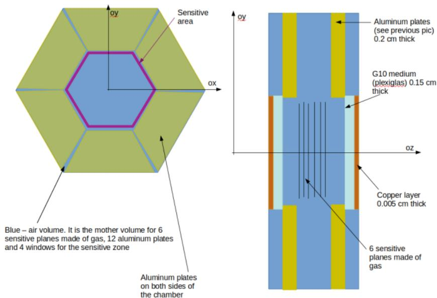
Figure 4. Schematic view of the MWPC detector
