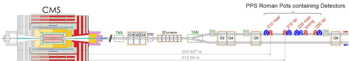
Figure 1. Schematic layout of the beam line between the interaction point and the location of the RP stations in the LHC (one side only).
