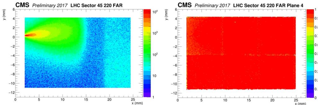
Figure 2. Left: impact point of the reconstructed tracks in a RP equipped with 3D pixels. Right: efficiency of a single pixel plane at the beginning of the data taking period in 2017.
