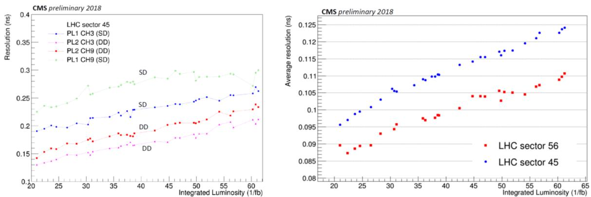
Figure 3. Evolution during 2018 data taking of the single channel timing resolution (left) and of the average time resolution from the track reconstruction in each of the timing RP (right).
