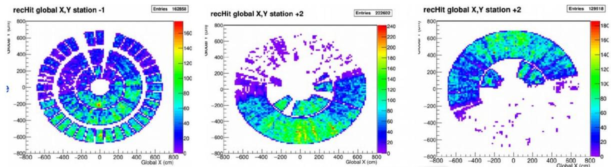
Figure 6. The hit occupancy in station ME-1 during a global run, including the upgraded ME-1/1 chambers (left). The 2 missing wedges were not included in the data taking for this run. The hit occupancy in station ME+2 during a global run, triggering on the bottom (center) and top (right) part of the detector and including the upgraded ME+2/1 chambers. The missing ME+2/1 chambers were not timed in at the time
