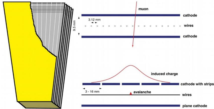
Figure 2. A CSC with 6 layers, with the radial cathode strips and transverse anode wires (left) and the schematic view of a gas gap showing the induced charge by a traversing muon
