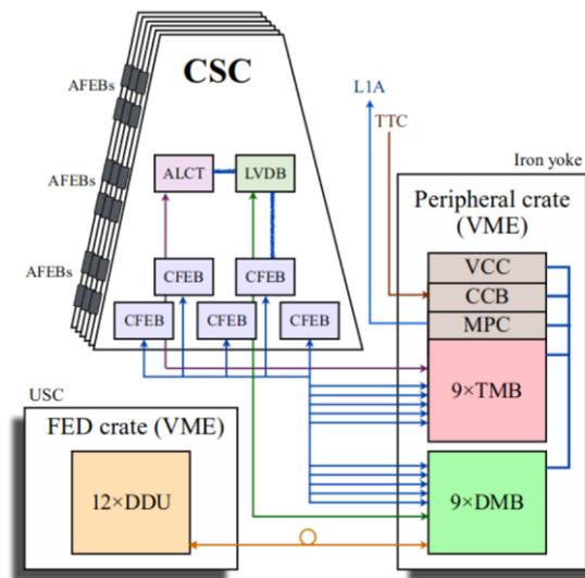
Figure 3. A schematic overview of the CSC electronics showing the boards located on the chamber, away from the chamber in the peripheral crate, and in the CMS service cavern (USC)
