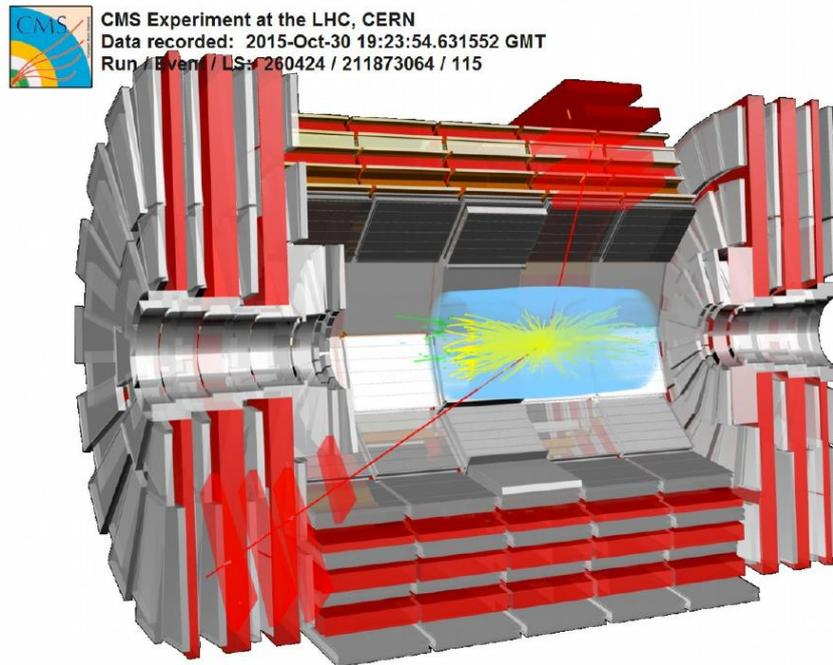
Figure 1. An event display showing two muons traversing the CMS detector. One of the muons is passing through cathode strip chambers in the endcap on the left
