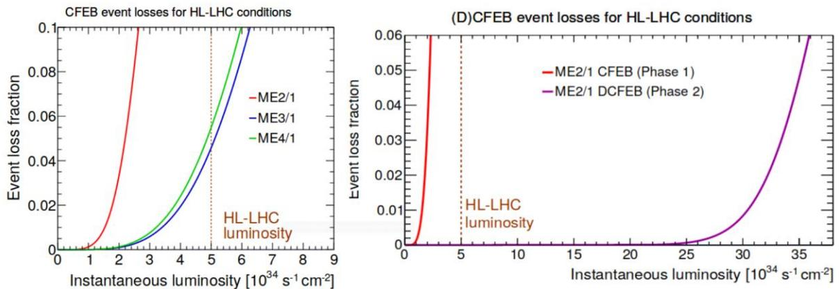
Figure 5. The expected event loss fraction in the ME2/1, ME3/1 and ME4/1 rings with the current CSC electronics as a function of the instantaneous luminosity (left) and a comparison to the expected event loss fraction with the new DCFEB (right)
