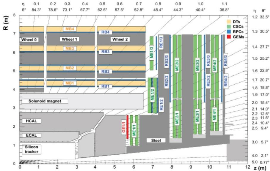
Figure 4. Schematic view of a quarter of the CMS detector showing the location of the different stations and rings of CSCs in green
