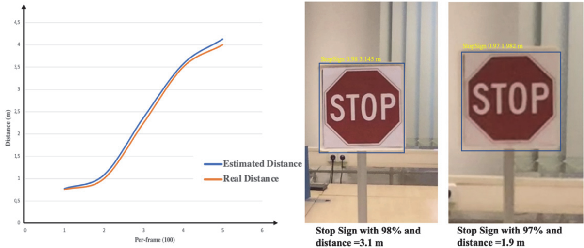
Figure 8 – shows the error rate between the estimated distance (blue line) actual distance (red line)
