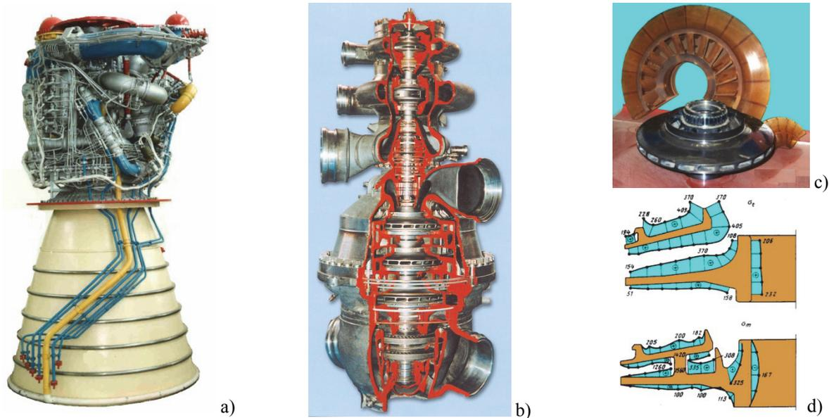
Figure 7 – Experimental study of the stress-strain state of the components of liquid-propelled rocket engine (a) and its turbo pump unit using the pump disk model (c) and data on stress distribution (d)
