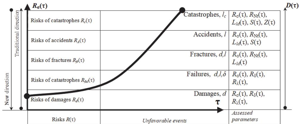
Figure 3 – Sequence of analysis of hazardous conditions of facilities and corresponding risks
