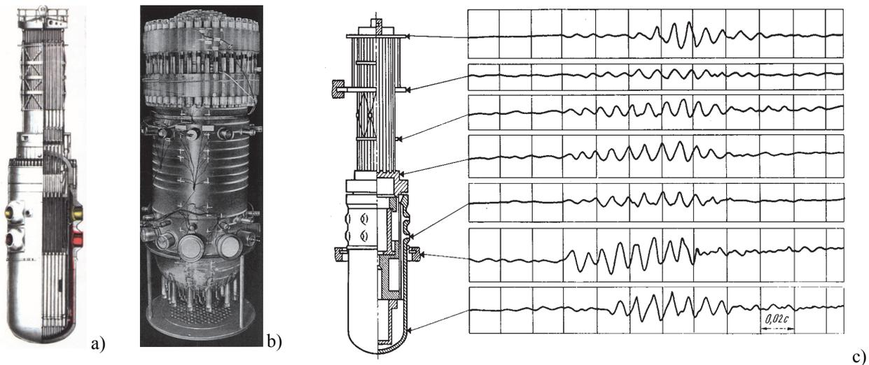
Figure 8 – Experimental study of the dynamics of a water-water energetic reactor (a) elements on its model (b) with registration of response diagrams (c)
