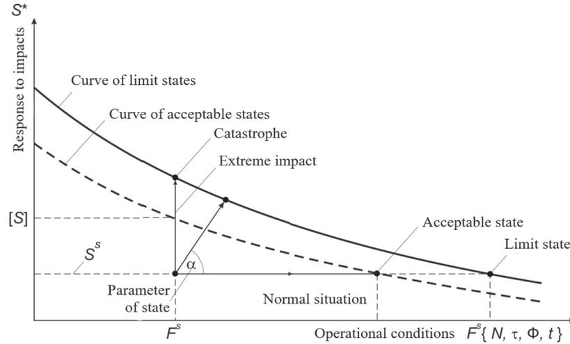
Figure 5 – States, scenarios and factors of operation of facilities with the possibility of accidents and disasters
