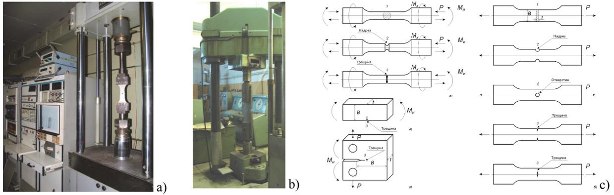
Figure 6 – Testing of samples (a) and full-scale models (b); types of test specimens (c)
