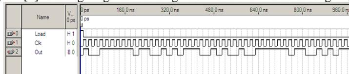
**Fig. 8.** Time charts of the barker-like code the dimension of which is  $N=28$ .
