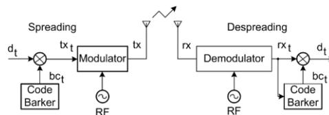
Fig. 2. The figuration of the functional scheme of the DS-SS system.
