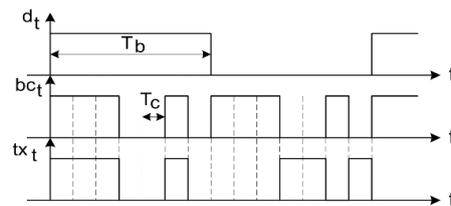
Fig. 1. The extension of the signal spectrum Barker code whose length is  $N=7$ .
