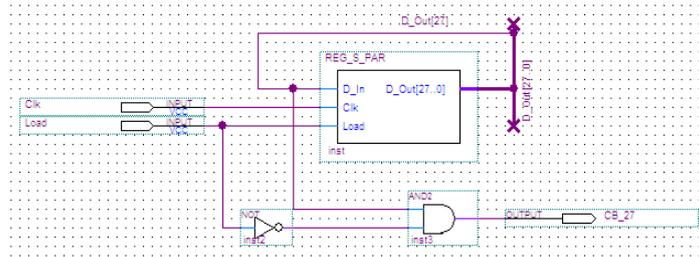
**Fig. 6.** Figuration of the barker-like code generation scheme ( $N=28$ ).
