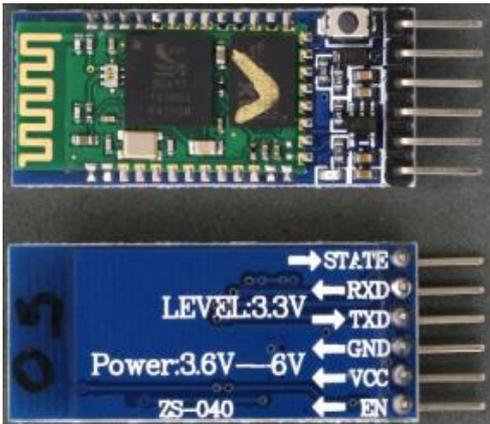
Fig 3. Front and Back view of HC-05 Bluetooth module [29]
