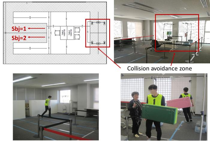
Fig. 2: Setting of the *in-vitro* experiment. Top left: the plant of the indoor controlled environment, where a  $U$  path has been defined. The collision avoidance zone is identified by a red rectangle and depicted also in the image at the top right. The two obstacles are controlled by one of the experimenter and the two subjects have to avoid the collision (figure bottom right). During the rest of the  $U$  path, subjects walk with their own natural pace.
