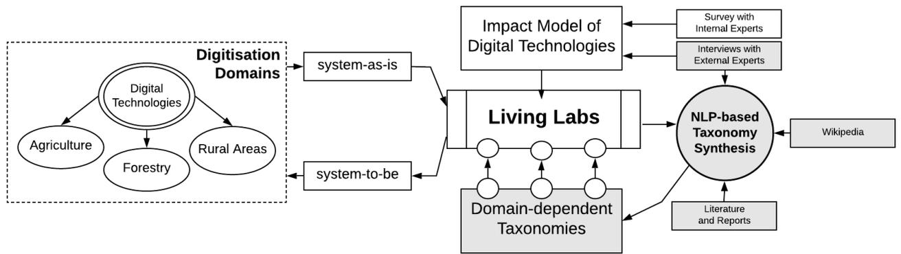
Figure 1: Overview of the DESIRA Project. The NLP-based part of the project is colored in grey (for “Interview with External Experts”, transcripts of the interviews are used as input for the process of NLP-based Taxonomy Synthesis).
