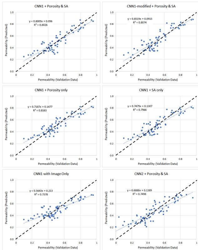
Figure 4. Comparison of the permeability prediction with six different models listed in Table 1 for the validation data. The linear regression fitting is also shown. The black dot line represents the perfect predicted case.
