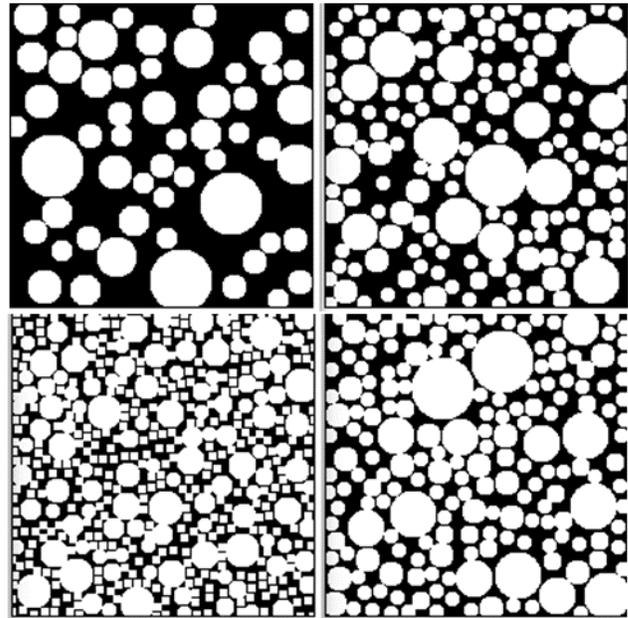
Figure 1. Examples of porous media generated with different sizes of sphere. Fluid flows through the void space in black. The black and white pixels have one and zero values in a Boolean type, respectively. Permeability decreases from upper left to lower right and ranges over two orders of magnitude in  $m^2$ .
