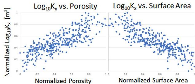
Figure 2. Normalized permeability in x-direction ( $\log_{10}K_x$ ) vs. porosity (left) and surface area.
