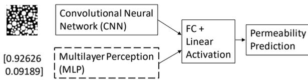
Figure 3. Schematics of convolutional neural networks and additional information stream to construct a physics-informed model architecture.
