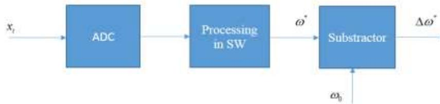
**Fig. 3.** Block diagram of frequency detector based on frequency estimator in sliding window
