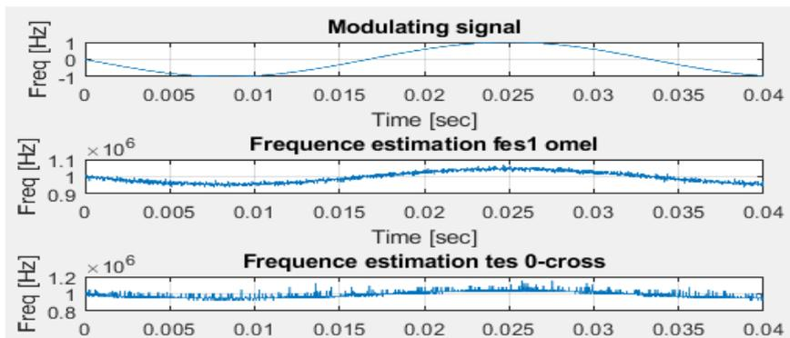
**Fig. 5.** Simulation of frequency detectors based on frequency estimator and 0-section counter in sliding window ( $n = 200$ ) with noise. SNR = 11dB
