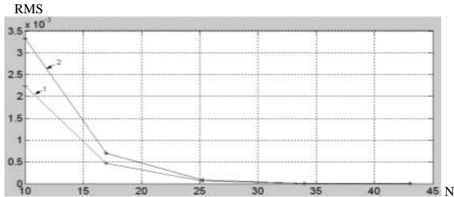
Fig. 9. RMS of the DDM assessment when changing the signal sample
