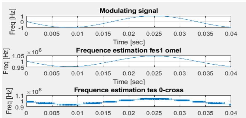
**Fig. 4.** Simulation of frequency detectors based on the frequency estimator and 0-section counter in a sliding window ( $n = 200$ ) without noise
