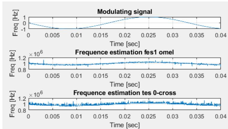
**Fig. 7.** Modeling of frequency detectors based on frequency estimator and 0-section counter in sliding window ( $n = 200$ ) with noise. SNR = 11dB and impulse interference with parameters: RMS HIP = 5V, probability of HIP action  $p = 0.001$ .
