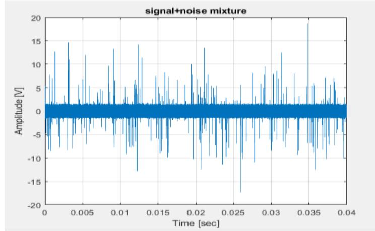
**Fig. 6.** Implementation of a mixture of FM signal, Gaussian noise and chaotic impulse interference. SNR = 11dB, RMS HIP = 5V, probability of HIP action  $p = 0.001$ .
