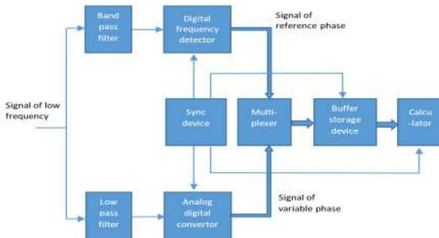
**Fig. 1.** The block diagram of the digital signal processing path implemented in the on-board navigation equipment VOR-85-01.
