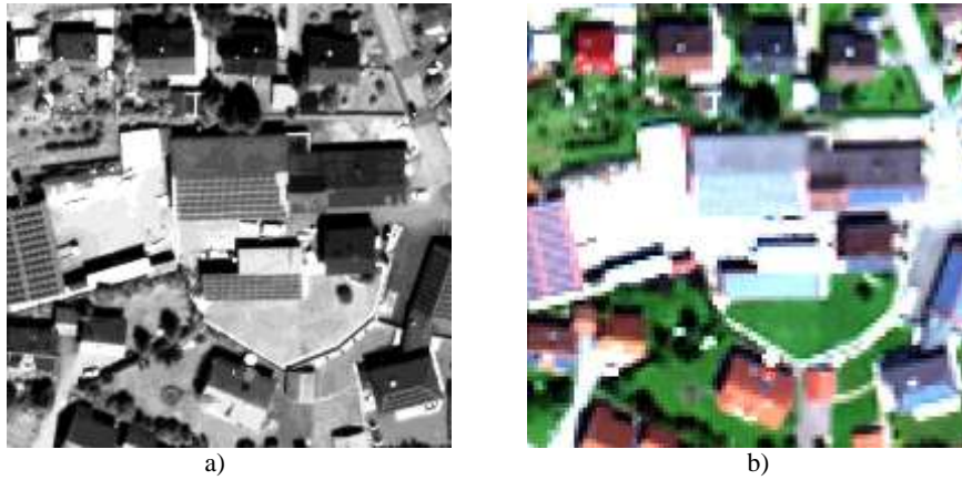
Fig. 2. Satellite images of WorldView-2: a) panchromatic; b) multispectral
