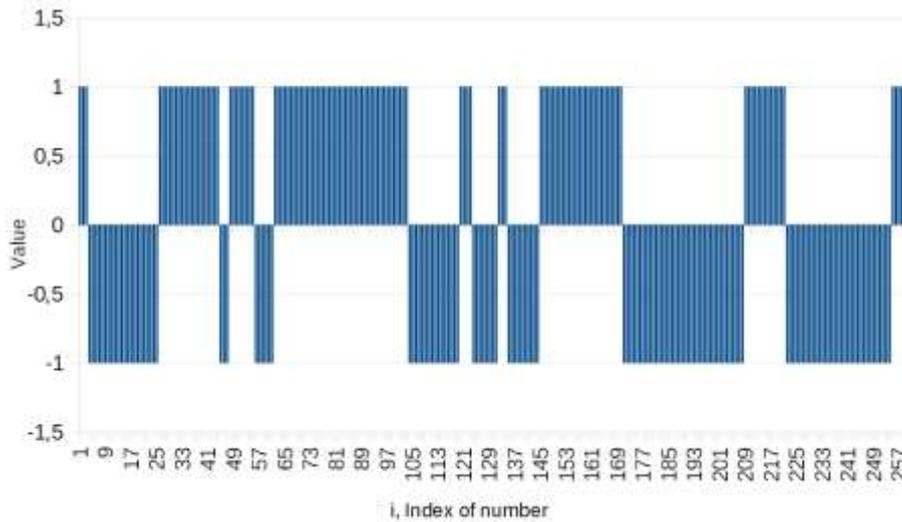
Fig. 7. Histogram of the signal obtained by generator with  $\lambda_0 = \lambda_1 = 0.05$ .
