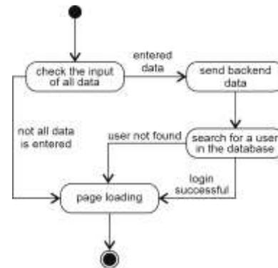
Fig. 3. UML state diagram for checking the input data
