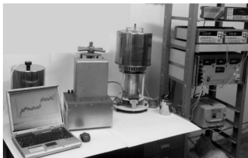
Fig. 6. Implementation of the hardware part of the heat flux density standard
