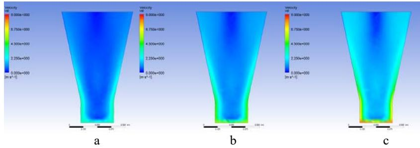
**Fig. 9.** The impact of granulator workspace design and gas flow velocity components on the gas flow total velocity and gas movement trajectory (working space "diffuser" with cylindrical insertion in the lower part),  $d=300$  mm;  $l_c=200$  mm;  $L=1000$  mm,  $\varphi=12^\circ$ : a -  $V_r=V_z=1$  m/s;  $V_\varphi=3$  m/s; b -  $V_r=V_z=1$  m/s;  $V_\varphi=5,2$  m/s; c -  $V_r=V_z=1$  m/s;  $V_\varphi=8$  m/s.
