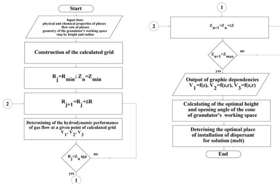
**Fig. 12.** An algorithm for vortex granulator hydrodynamic calculating
