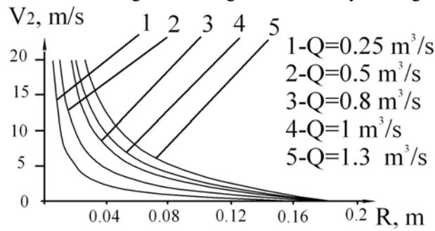
**Fig.5.** Calculated change of the radial velocity of the gas flow.
