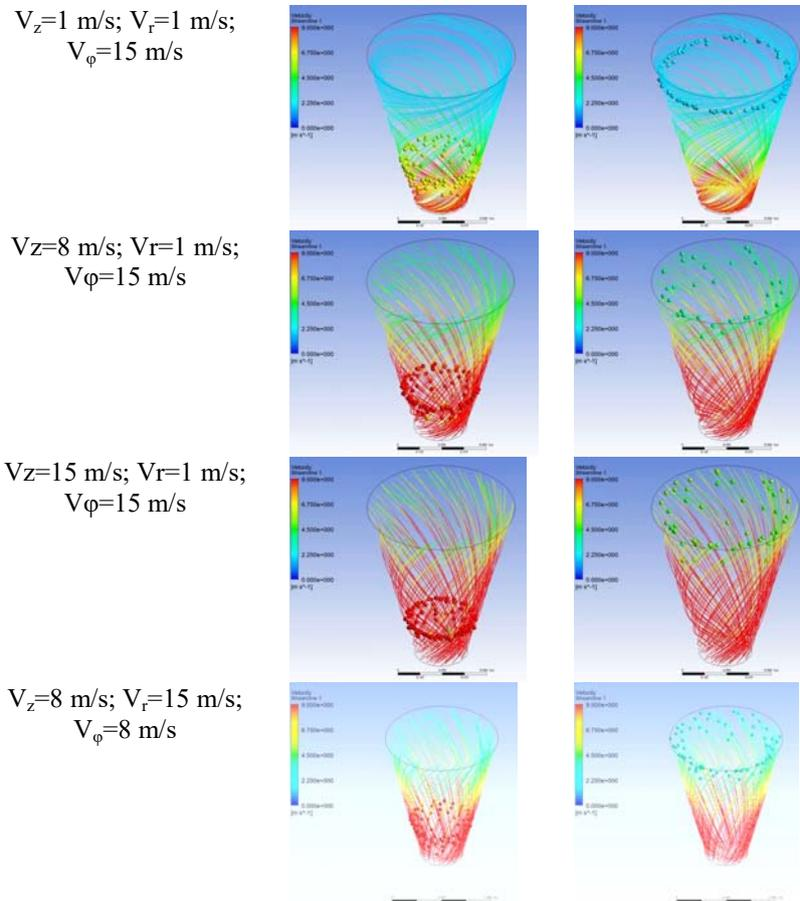
**Fig.11.** Gas flow movement trajectory for different values of speed components.
