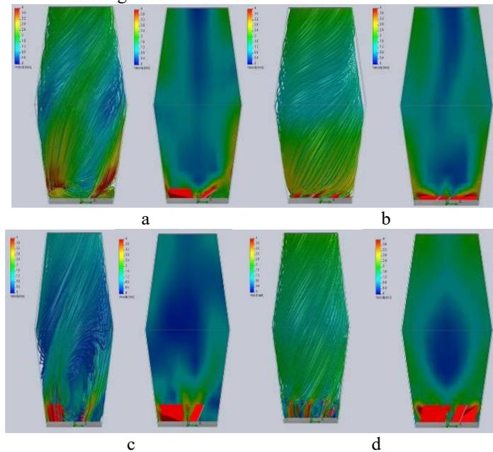
**Fig. 8.** Filling the gas flow velocity field when installing of gas-distributing unit with blades: a –  $\alpha=30^\circ$ ,  $n=3$ ; b –  $\alpha=30^\circ$ ,  $n = 8$ ; c –  $\alpha = 60^\circ$ ,  $n=3$ ; d –  $\alpha=60^\circ$ ,  $n=8$ .
