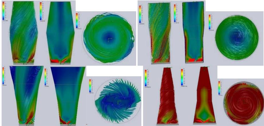
**Fig. 7.** Filling the gas flow velocity field when installing of gas-distributing unit with blades and various configuration of granulator workspace with blades inclination angle  $\alpha = 30^\circ$  and their number  $n = 3$ .
