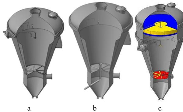
**Fig. 14.** Vortex granulator designs: a – with spraying of the melt; b – with a previous wetting of granules and simple inner case; c – with separating device for exhaust gases cleaning
