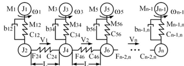
**Fig. 1.** Kinematic diagram of a multi-mass interconnected system taking into account elastic bonds of the first and second kind
