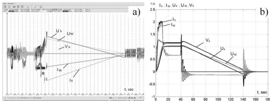
**Fig. 9.** Average CRM electromechanical processes (a), simulation results (b) in case of a strip break
