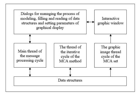
Fig. 1. BLSD CAD-system architecture
