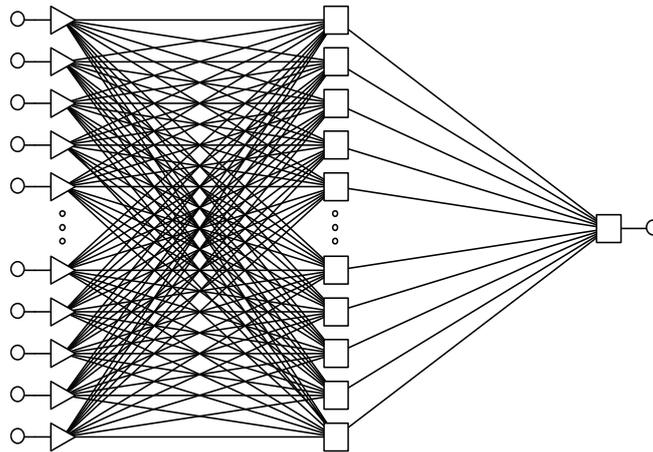
**Fig. 7.** MLP 15-12-1 Three-Layer Perceptron Architecture with Logical Signal Transmission for Time Series Prediction of Globe Seismic Monthly Dynamics ( $N_{\Sigma}(t)$ ) (Source: author's own elaboration)
