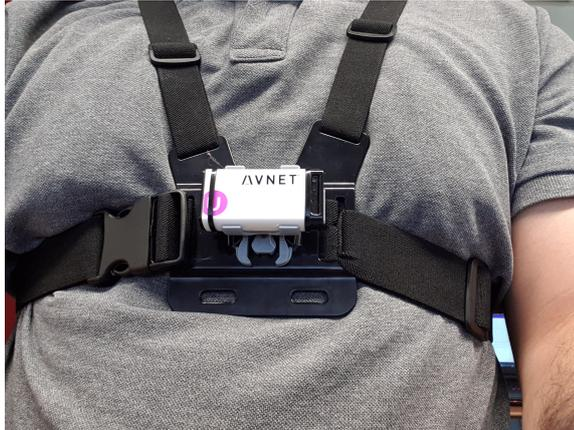
Fig. 2: Harness with AVNET sensor.
