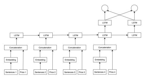
Fig. 3: A demonstration of the stacked LSTM structure. In this example, it uses data of four days to predict the gas price of the next two days
