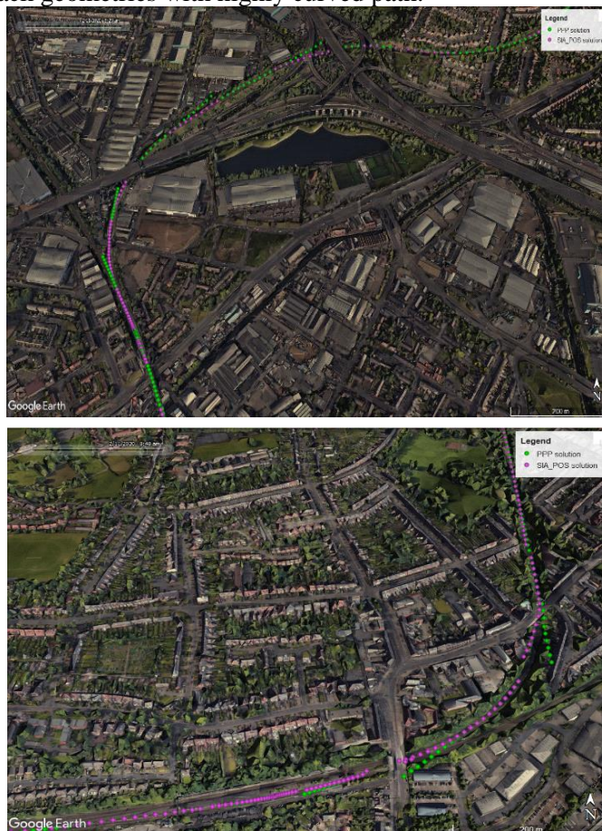
Figure 5: PPP (green) and SIA_POS (SIA_POS) trajectories over two curved sections of the tracks having 10s measurement gaps every 20s.
