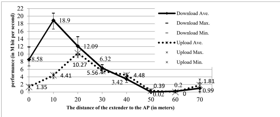
Fig. 4. The Extender Performance as Download and Upload Speed of the Extender line graph
