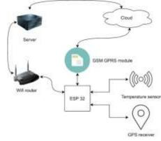
Fig. 2. Schematic diagram of the system for clarifying the temperature of potentially "sick" people
