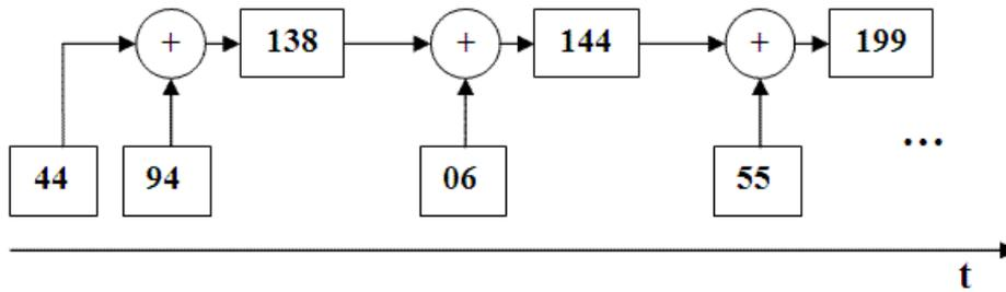
**Figure 3.** Sequential summation with  $\Delta t_{\text{dat}} \geq \Delta t_{\text{add}}$
