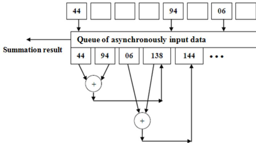
Figure 2. Summing asynchronously input data
