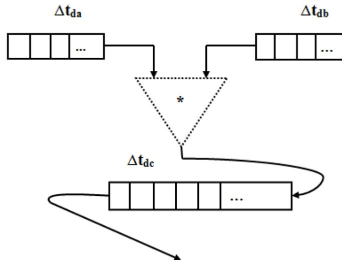
**Figure 5.** Asynchronous computing diagram at the decomposition stage of solving the problem of pairwise multiplication of two vectors
