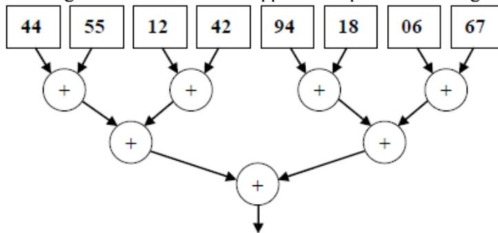
**Figure 1.** The cascading scheme of addition vector elements
